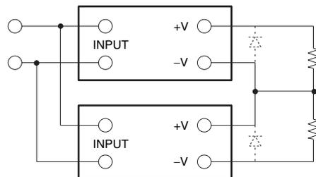
When connecting the Power Supplies in series with an operation amplifier, connect diodes to the output terminals as shown by the dotted lines in the figure. No diodes are required with S82K-□09024 and S82K-□10024.
