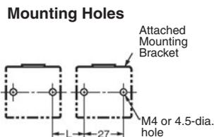
Note: If more than one Power Supply is installed in a row, keep a distance of 20 mm min. (L = 20 mm min.) between each adjacent Power Supply.
