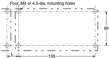
**Note:** If more than one Power Supply is installed in a row, keep a distance of 20 mm min. (L = 20 mm min.) between each adjacent Power Supply.
