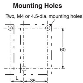
Note: If more than one Power Supply is installed in a row, keep a distance of 20 mm min. (L = 20 mm min.) between each adjacent Power Supply.
