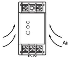
When mounting two or more Power Supplies side-by-side, allow at least 10 mm spacing between them, as shown in the following illustration.
