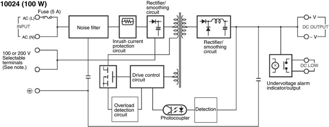
**Note:** Use the short bar to short-circuit terminals 7 and 8 to select 100 to 120 VAC and remove the short bar to select 200 to 240 VAC.
