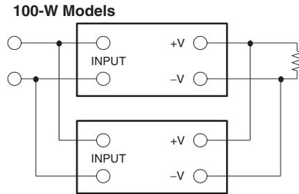
**Note:** When operating the S82K-P10024 in parallel operation, set the selector to "PARALLEL". In this case, the rated current per S82K-P10024 is 3.78 A.
