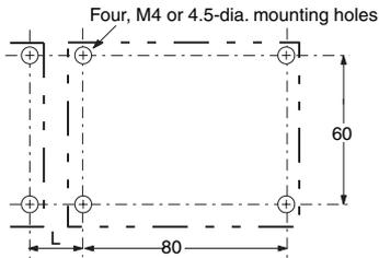
**Note:** If more than one Power Supply is installed in a row, keep a distance of 20 mm min. (L = 20 mm min.) between each adjacent Power Supply.
