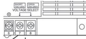
Remove the short bar to open terminals 7 and 8.
