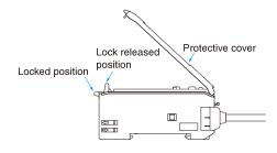
Note: 1. To maintain the fiber characteristics, make sure that the lock is released before removing the fibers.
