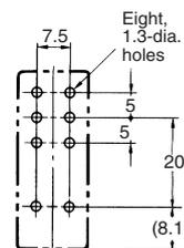
**Mounting Height of Relay with Back-connecting Sockets**
