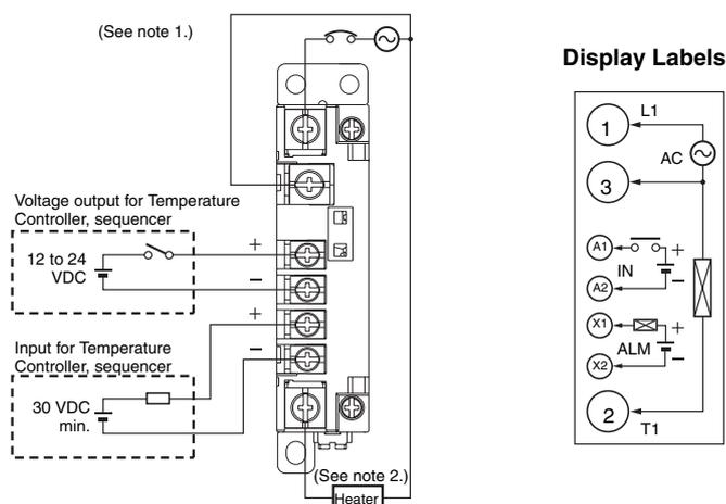
**Note:** 1. If the detection power supply terminal (terminal 3) is not connected, failure detection is not performed and so be sure to connect this terminal.
