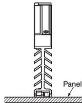
**Note:** Use the G3PC at a load current of 50% of the rated load current when it is mounted horizontally.
