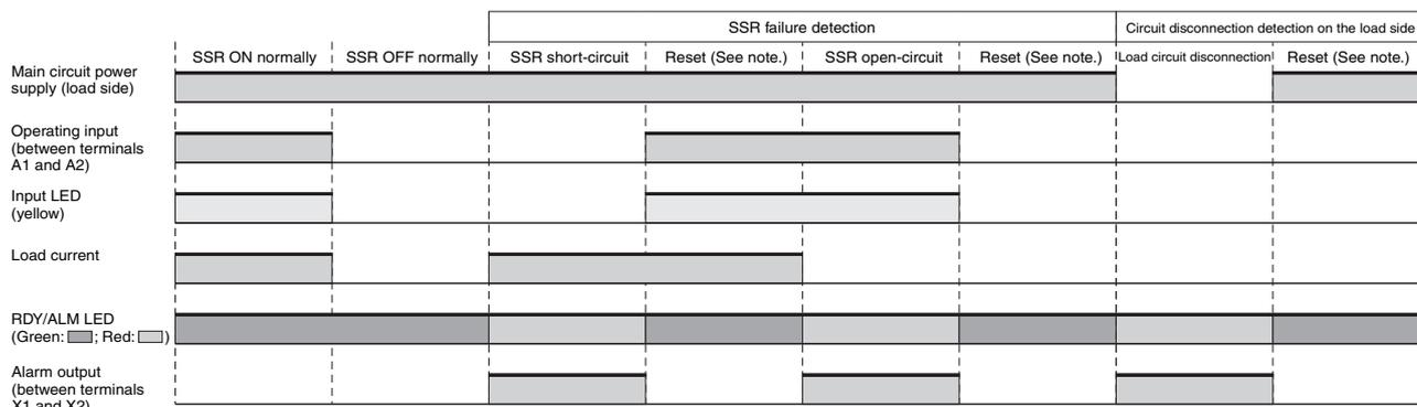
**Note:** After failure detection, if the detection conditions differ to the conditions given under *Conditions for SSR Failure Detection*, alarm output is reset.
