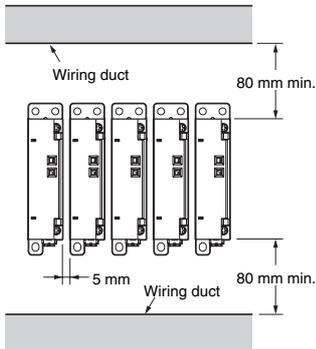
**Note:** Use the G3PC at a load current of 80% of the rated load current when it is mounted side by side.
